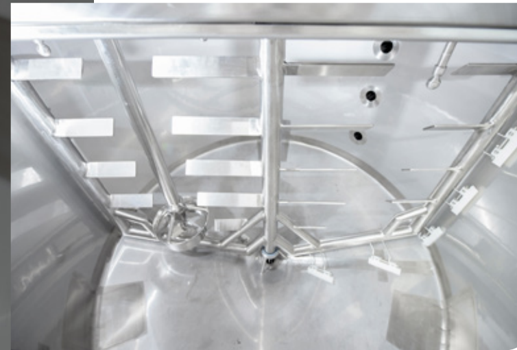
Jetstream mixer with anchor agitator
